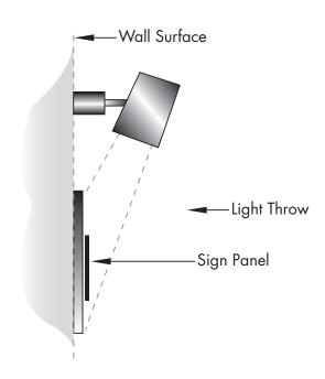
Lighting source may include fluorescents or LED's and various forms and shapes. Specific lighting components are not strictly specified. Designs shall be approved by the owner.
